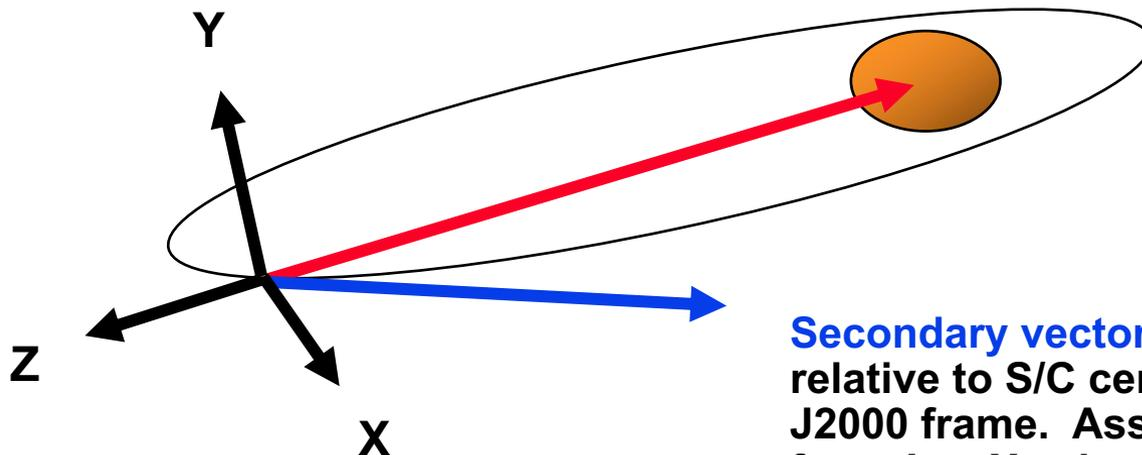
**Primary vector:** spacecraft nadir direction vector. Aligned with nadir frame's -Z axis.
