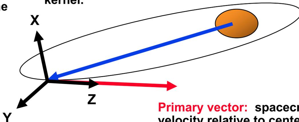
Normalized component of secondary vector orthogonal to primary vector is aligned with the view frame's +Y axis. ("In plane" direction)
