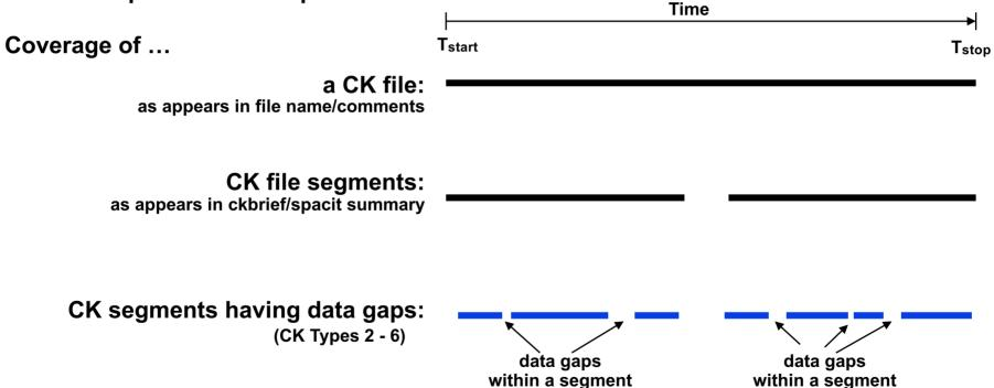
The blue line segments represent interpolation intervals – times when pointing will be returned. For attitude requests within gaps, high level SPICE APIs will signal an error.
